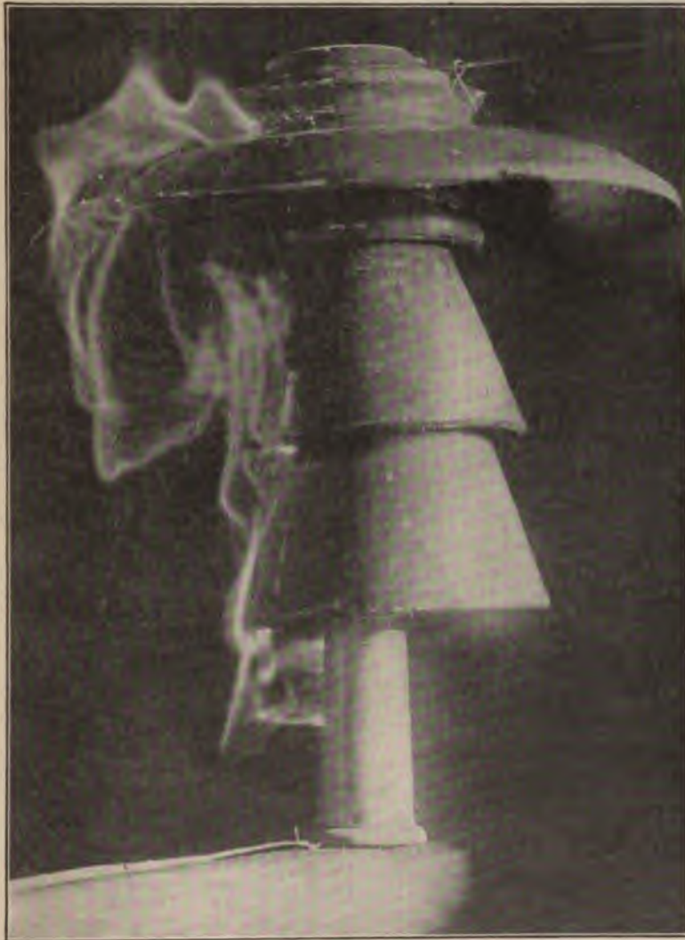
INSULATOR. ARC TO METAL PIN AT 96,000 VOLTS. Precipitation \frac{3}{4} inch per minute. Diameter 14". 30° above horizontal. Height 12". Duration of test, 15 minutes. Weight 22 lbs.
